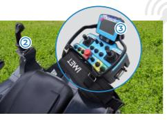
Driving position with ROPS / FOPS approved canopy, reclining and longitudinally adjustable padded seat. In onboard driving mode, the travel and lift operation controls are transferred to an **ergonomic proportional joystick** that allows precise control of the machine.
